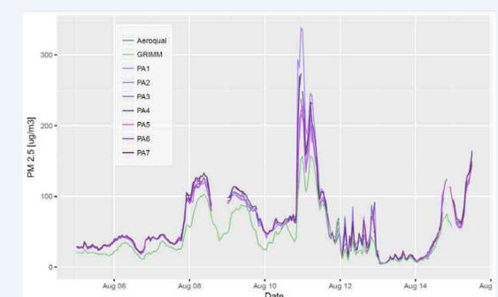
Figure 6: Hourly uncorrected data from August 2018 showing increased PM<sub>2.5</sub> concentrations recorded by multiple small sensors and GRIMM monitor during a significant smoke event in Edmonton, AB.
