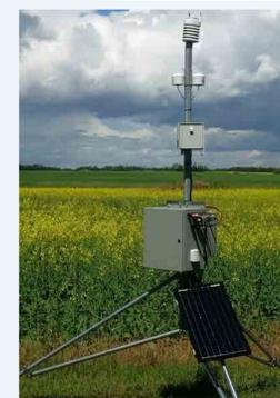
Figure 4: Self-contained tripod deployed SW of Edmonton containing PurpleAir sensors, Aeroqual AQY, 2B OEM-106L and Vaisala WXT with solar/battery power.
